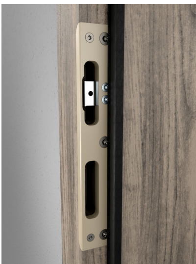
Caption text: Enabling the adjustment of rebated doors from the striking plate side: The new "Stabilo striking plate 28 2-Hole" with a solid construction. A U-shaped stainless-steel profile with which the contact pressure of the door seal can be adjusted is fitted in the top aperture. Photo: Basys
