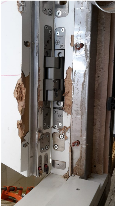
Photo 2: The "Pivota DXS 300 3-D" is capable of supporting 350 kilograms per pair and made entirely of steel. This gives the hinge an RC4 break-in resistance class. The picture shows the hinge after passing the break-in test. Photo: Huber Form Schreinerei GmbH, Triftern-Neukirchen
