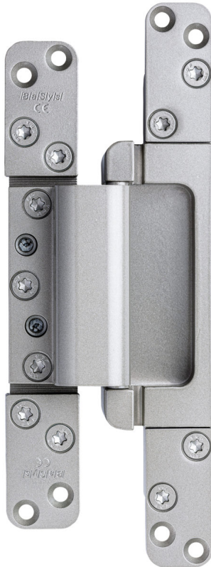
Caption 1: BaSys is moving the side gap adjustment to the frame part of the hinge "Masterband FX2 120 3-D FD" developed for rebated front and apartment doors with an 18 mm overlap and leaf seal. This ensures that the tightness of the door is maintained during adjustment. Photo: BaSys
