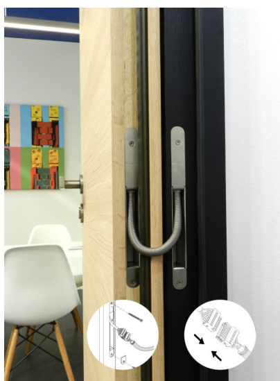
Caption: The "Pivota Connect" cable connector disappears into a milled groove in the door rebate and secures the power supply between the frame and door leaf - a prerequisite for equipping the door with additional security and convenience features. Now the system is also available with plugs. Photo: Basys
