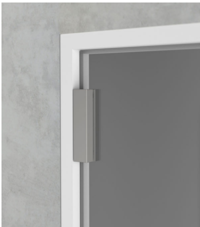
Caption: Basys developed a concealed hinge for glass doors. The frame part disappears into the frame and a door part is hidden from view in a casing attached to the glass door. Photo: Basys
