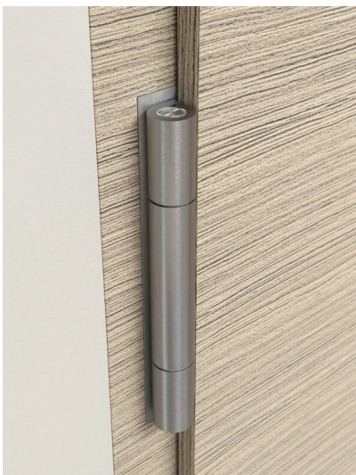
Caption: The new "Objecta 2039/160/56-4" for rebated doors is slimmer with a barrel diameter of just 20 mm, but like the "2239" it can also carry doors weighing 300 kilograms. There is also a variant for continuous seals in the door leaf and a version for flush doors. Photo: BaSys
