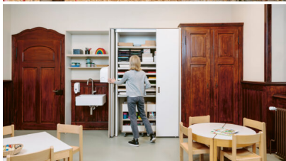
Caption 2: Nolè - Schneeberger Architects complemented the historic elements with understated cabinet elements with front panels that can be opened all the way without causing an obstruction by disappearing completely into a side pocket, therefore saving space. Photo: Hawa Sliding Solutions AG
