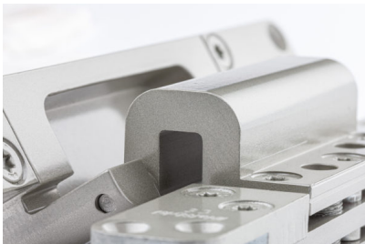
Caption 3: The "Masterband FX2 120 3-D FD" has already received one of the coveted "Winner" awards at the German Design Award. It has a load-bearing capacity of 120 kilograms per pair, maintenance-free bearings and three-dimensional adjustment - recently without any negative effects on the tightness of the front door. Photo: BaSys
