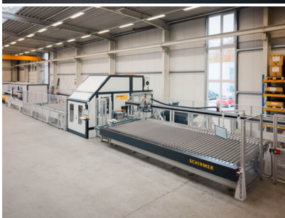
Caption 3: A customer-specific through-feed fab centre configured for Bosch Rexroth for processing aluminium construction profiles. Photos: Schirmer Maschinen
