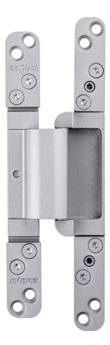
Caption 1: In the well-known "Pivota FX2 60 3-D" for rebated standard interior doors, the side gap adjustment was still in the leaf part of the hinge. When adjusting the side gap, it happened that the leaf-side hinge body slid out of the door rebate. Basys has optimised the product and discontinues production of this old model. Photo: BaSys
