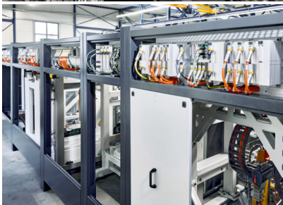
Caption 4: Schirmer is switching completely to the pluggable 'MX' system solution from Beckhoff Automation for the automation of its machines. It completely replaces the control cabinet. Photo: Beckhoff Automation
