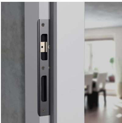
Caption: Being able to adjust doors from the striking-plate side: The new „Stabilo striking plate 28 2-hole light V2“. In the top aperture it's fitted with a U-shaped stainless-steel profile, that increases or reduces the door seal's contact pressure. Photo: Basys
