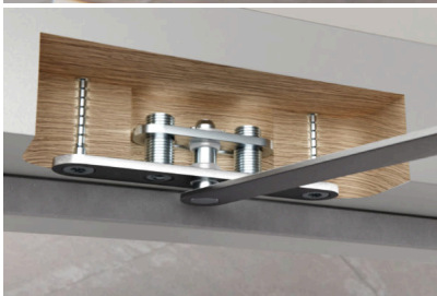
Caption 3: In contrast to other similar products, the new opening angle limiter does not restrict the height adjustment of the door; the counter bearing in the frame is also height-adjustable and moves with the adjustment. Photo: Basys
